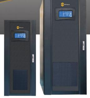
The HT5000T series is available from 20kVA to 120kVA models Model HT5000T monitoring and control data are shown on an easy to understand front panel display with LCD 5.7 inches touch featuring pushbutton controls, LCD read out for event logs and diagnostics and a mimic diagram for system status. The power protection system can be remotely monitored via RS232, RS485, dry contact or SNMP interface.
